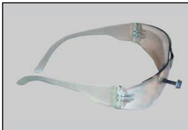
The screw went straight into the lens, but no metal went through.
